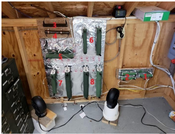
Figure 5. Resistor sets used in study, red number correlates with resistor set number, Appalachian State University State Farm Solar Lab.
